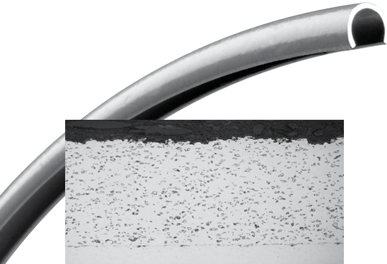
Figure 1: TriCom is a composite coating consisting of a cobalt matrix with chromium-carbide reinforcing phase.
